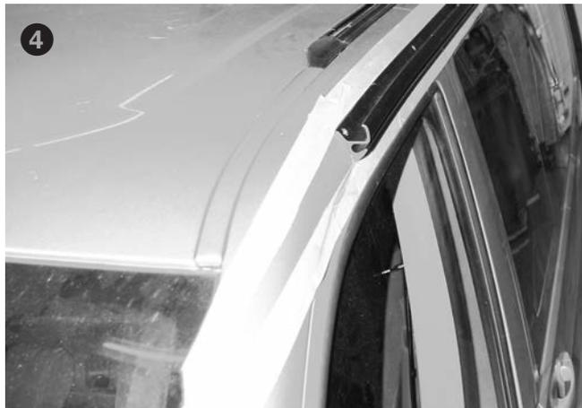
Equally attach masking tape to the vehicle sheet above and beneath the front spoiler (cp. image 4, 5).
