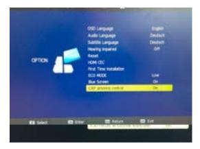
When you turn off the TV set (Stand-by), the KATHREIN antenna control will ask whether the antenna should remain extended or whether it should retract.
