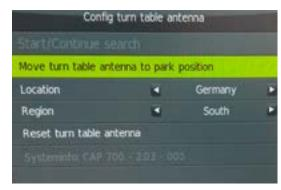
If the alphatronics TV is to be operated with a domestic system or multi-switch, you can turn **OFF** the**KATHREIN antenna control** in the last row using the arrow keys.
